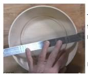
To layout the cut, he first determines the best grain orientation, realizing also that the front of the finished piece will actually be the bottom of the small section removed. He marks the center line at the rim.
