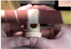
Use the sanding stick to sand open an access hole in the side of the piston. Clean up the hole with hand sanding. Hand sand the piston to get the desired fit of the piston into the body.
