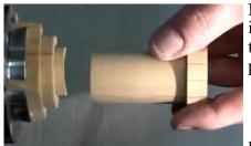
Now clean up the end of the blank once again and create a short tenon to fit into the open end of the piston tube. Leave enough room for glue between the joint. Sand the end of the tenon as this will be the inside bottom of the piston.
