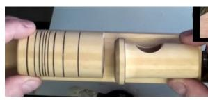
The layout of the box in the blank is shown on the left. The body of the box is on the left half of the picture, with it's open end facing the tailstock. The piston insert is on the right half of the picture, with it's lid on the left and bottom closest to the tailstock on the right.
