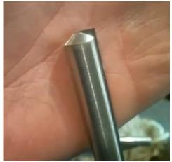
Another way to refine the shape is to use what Trent call a "clean cut tool", shown to the left. It's a 1/2 inch bowl gouge ground straight on the right side, and slightly swept back on the left.
