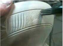
At left, Trent also demonstrated using a needle scaler. The scaler left an "orange peel" finish on the wood.
