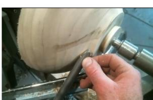
Trent uses a shear scrape to refine the profile. Drop the tool rest, lower the handle, and close the flute as shown on the left. The edge of the gouge should contact the wood at a 45 degree angle. Look for long stringy shavings, as shown below, as evidence you are making a good cut.
