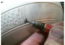
Shown on the left, he demonstrated a micro die grinder with a three sided rotary tool.
