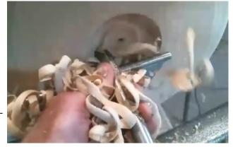
Now Trent removes the blank from the screw chuck and reverses the bowl to be held by the tenon. Just as he did on the outside, he takes successive cuts, practicing as he approaches the final shape.
