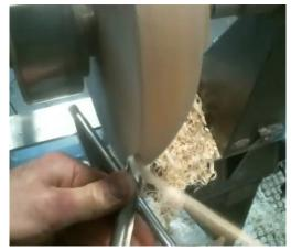
Trent now trues up the top of the bowl by cutting straight in from the left as shown. Cut in steps and establish what will be the top edge of the bowl. Use a scraping cut from center to outside edge to clean up.
