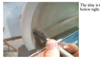
Trent uses the clean cut tool to clean up the inside of the bowl.
