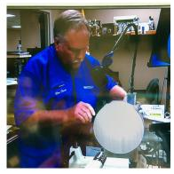
Ron Ford lead off the demonstration by turning an Ogee shaped platter. One thing to note was Ron used a glue block to hold his platter by the foot. He attached it with a piece of brown grocery bag sandwiched between the glue block and the platter, held in place with Titebond glue.
