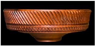
You can use a parting tool or a "three point tool" to separate or frame areas of embellishment. The bowl to the right is an example of using a parting tool between the spiral cut and knurled sections.
