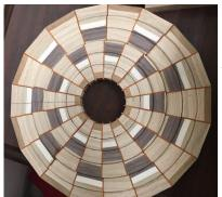
Transfer the "keystone" mark to the outside edge of each circle. This will serve as a visual reference as the layers are glued together to form the bowl blank.
