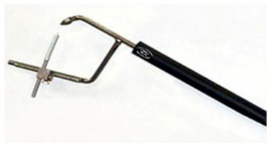
This is the Crabtree Hollowing King (shown to the left). It comes in five sizes depending on the size of your lathe and size of your blank. I would opt for a smaller version to start. If you like this system you can purchase larger ones or move on to a more robust system. This is the tool that I own.
