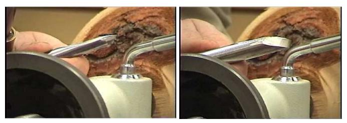
Keith explains the types of grinds he uses for his finishing cuts. The photo on the right is a spindle gouge with a free hand fingernail grind. The photo on the left is an Ellsworth bowl gouge with the grind sharpened with the Wolverine system. To get the fine tear-out free finishing cuts, sharp tools are a must.
