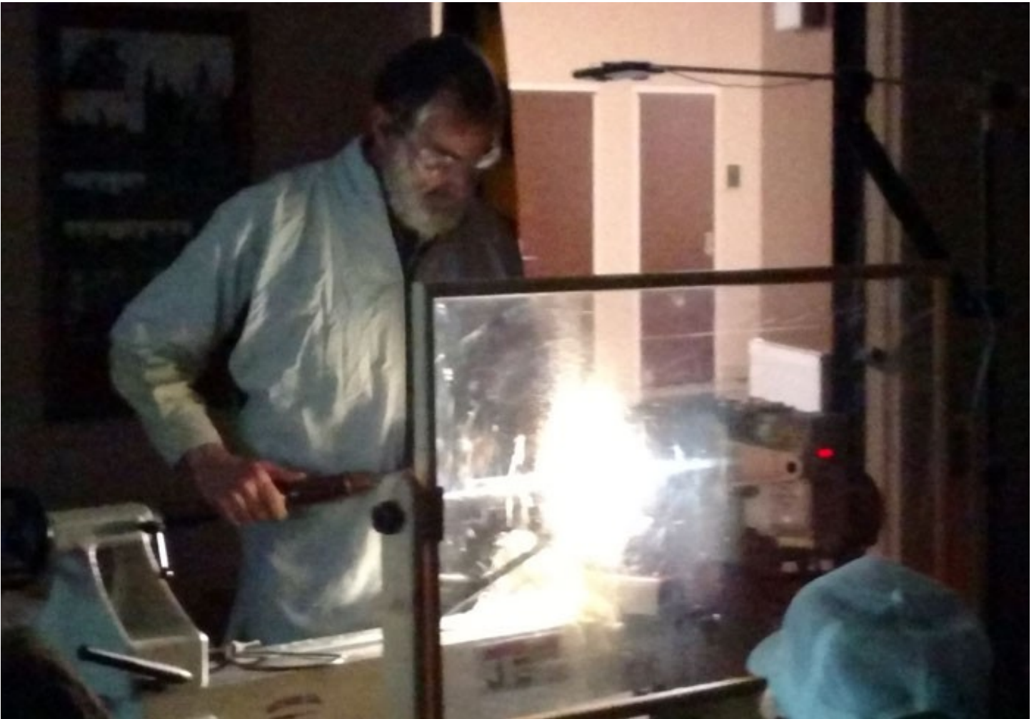
Joe works in the dark with just one lamp shining into the bowl to illuminate the wall thickness.
