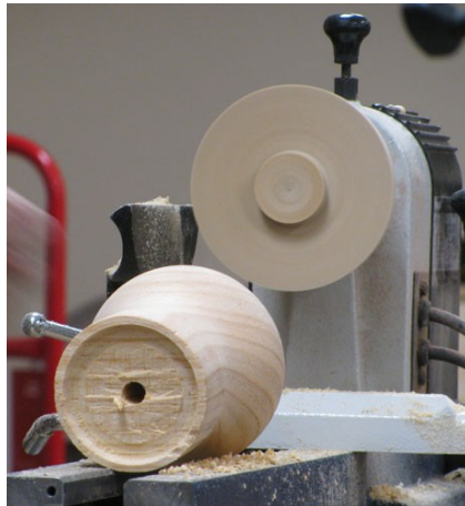
Chuck has sized the plug so that it will fit into the access hole in the base of the vase.
