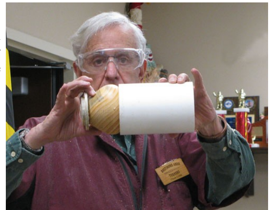
Reverse mounting the vase with the neck extended into the PVC pipe.
