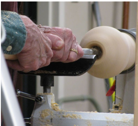
Hollowing the base of the vase thru the bottom access hole.
