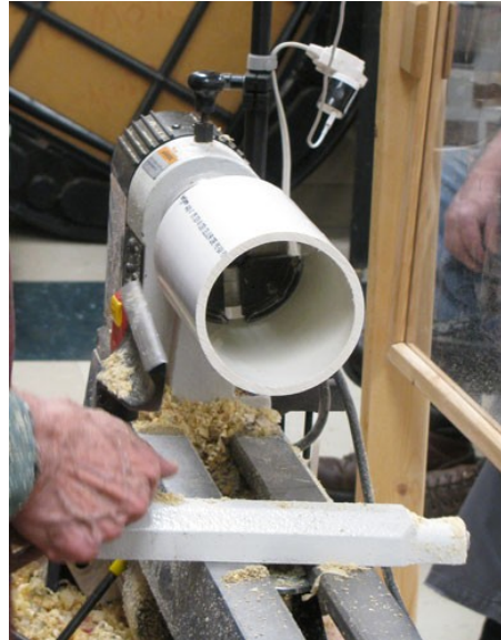
PVC pipe in the chuck for reverse mounting the vase.
