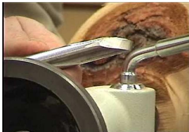
Keith explains the types of grinds he uses for his finishing cuts. The photo on the right is a spindle gouge with a free hand fingernail grind. The photo on the left is an Ellsworth bowl gouge with the grind sharpened with the Wolverine system. To get the fine tear-out free finishing cuts, sharp tools are a must.
