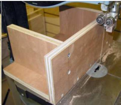
Saw slabs on well fenced bandsaw.
