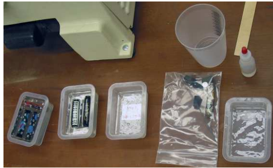
The stages of embedding a pen blank.
