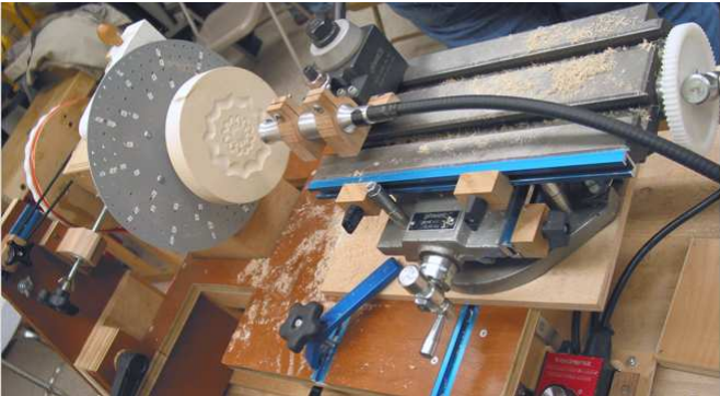
Dean Swaggert's home-brew Rose Engine in action. (Note the stops Dean added to the X-Y Table.)
