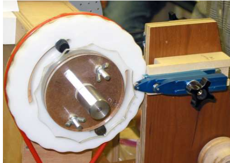
Rubber rubs rosette, deflecting lathe spindle.
