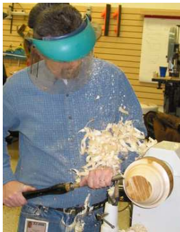
Wayne Kuhn spent much of the evening turning a bowl from a piece of green birch. (L->R) Shavings fly as he roughs the exterior; BAT members look on as he refines the profile; Mike Lang and Steve Lane give advice in hollowing.
