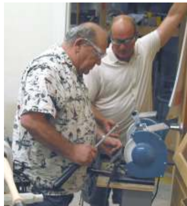
Lou Rudinski shows how to sharpen a gouge.
