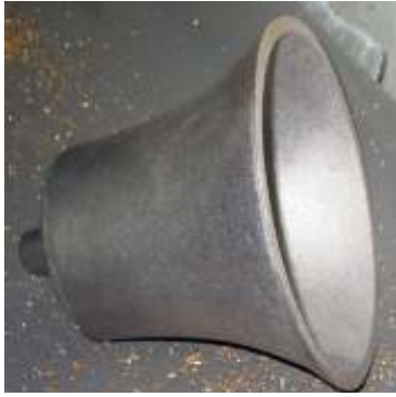
Bronze Casting as received from the foundry.
